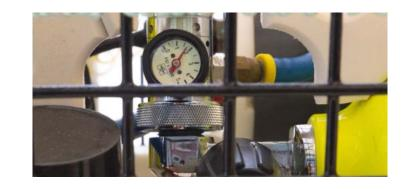
2) To remove the air tank, open the lid of the unit – unhook the bungee cord, open hinged lid, remove the white, grid-like section (it lifts right out).
