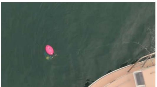
4) There's a tilt sensor in the unit and after a certain, specified time, it will stop releasing air into the bag. The bag will not explode because there's a relief valve on it. As it raises in the water, air is releasing from the bag.
