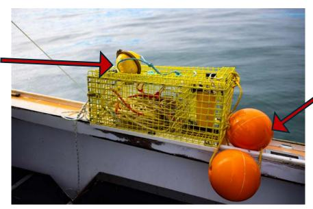
Orange buoys – connected to lid. When lid pops up, buoys float lid to surface.
