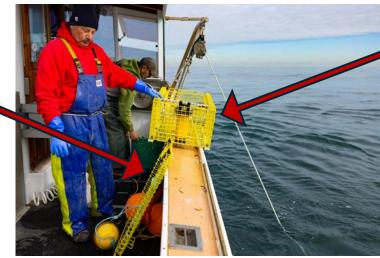
Cage – rope that connects lid to rest of unit is packed in here, as are the mechanical components
